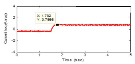
Figure7b: Current response of the PMSM with the proposed controller under increasing load.
