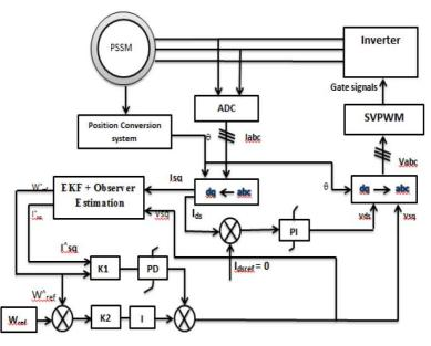
Figure 3: Experimental setup of PMSM speed controller.
