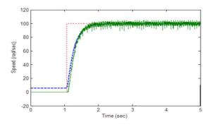
Figure4a: Speed response of the PMSM without the controller under no load.
