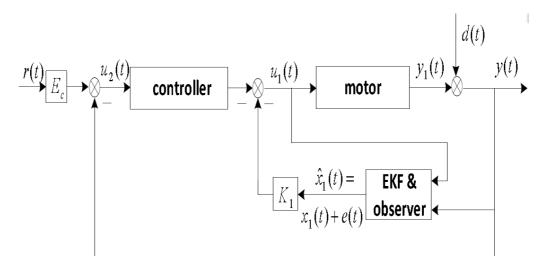
Figure 2: The block diagram of speed controller using the EKFcombined with the state observer.
