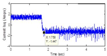
Figure 9a: Current response of the PMSM without the controller under decreasing load.
