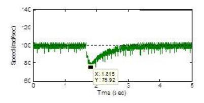
Figure6a: Speed response of the PMSM without the controller under increasing load.
