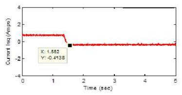
Figure9b: Current response of the PMSM with the proposed controller under decreasing load.
