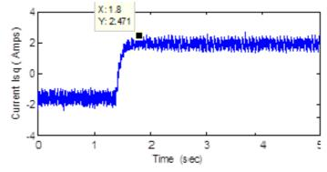
Figure 7a: Current response of the PMSM with the proposed controller under increasing load.
