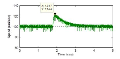
Figure 8a: Speed response of the PMSM without the controller under decreasing load.
