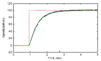
Figure5a: Speed response of the PMSM with the proposed controller under no load.
