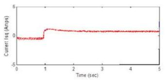
Figure 5b: Current response of the PMSM with the proposed controllerunder no load.
