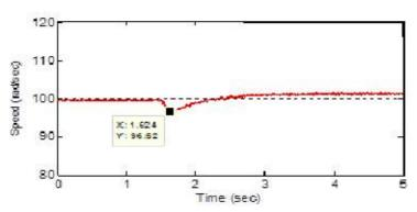
Figure6b:Speed response of the PMSM with the proposed controller under increasing load.
